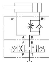
**3 MAIN CHARACTERISTICS OF MODULAR FLOW CONTROL VALVES TYPE WHQ, WKQ, WJPQ**
