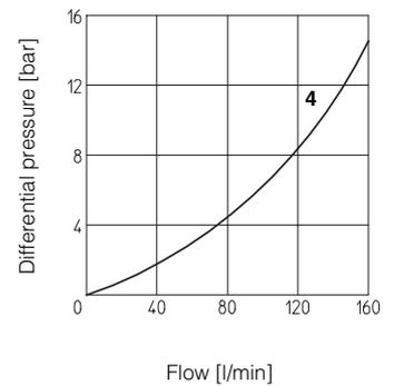
**6 DIAGRAMS OF WJPQ-2** based on mineral oil ISO VG 46 at 50°C
