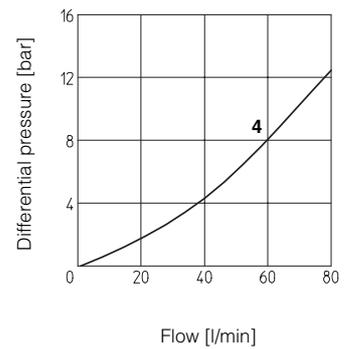
**5 DIAGRAMS OF WKQ-0** based on mineral oil ISO VG 46 at 50°C
