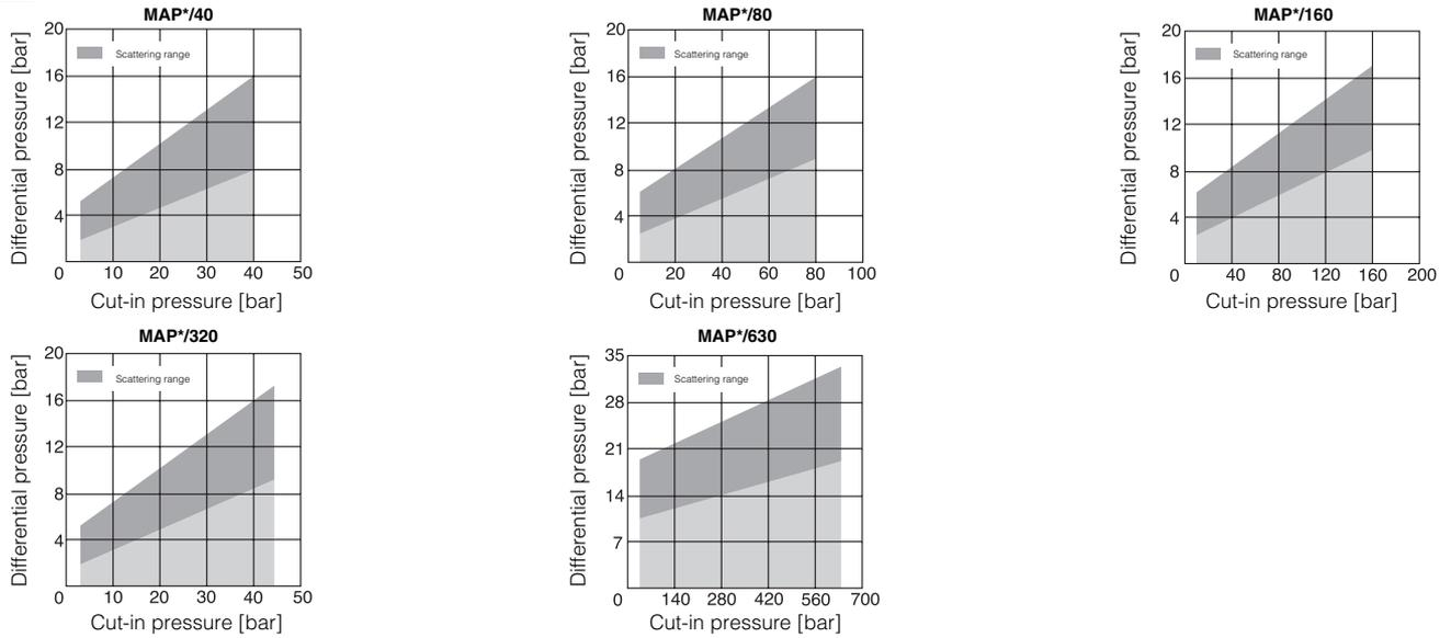
The graphs show, according to the set cut-in pressure, the pressure difference between the insert and the resting positions of the pressure switch electric contacts.
